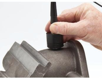
Many cast metal parts or sound-attenuating materials can be measured with the High Penetration software option.
