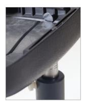
The standard probe along with one of the two target disks and a replaceable chisel wear cap makes the Magna-Mike 8600 gauge ideally suited for most automotive tear seam applications where measurements need to be made in a thin channel or groove.
