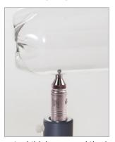
In applications such as plastic containers, simply drop the small target ball inside the container. The magnetic probe held on the outside of the container attracts the target ball. When scanning the probe along the surface or critical corners, the small steel target ball will follow. In the Minimum Mode feature, the gauge continually displays both the
